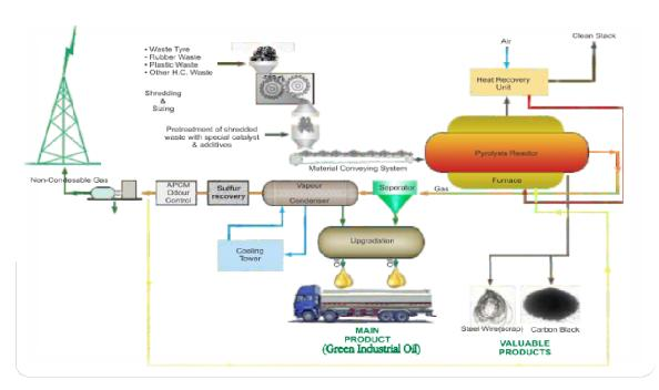
Pyrolysis of waste hydrocarbon (WHC)is not a combustion it is 100% conversion of waste hydrocarbon into valuable hydrocarbon. Technically it is the thermal catalytic de-polymerization of waste hydrocarbon in the absence of Oxygen(O2), Causing it to breakdown into materials that they were made of Generally WHC breaks into main three products.
